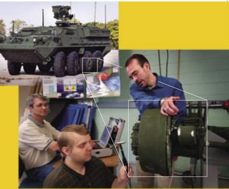
Douglas Adams, right, and research engineer Ronald Evans, left, with doctoral student Harold Kess, who's using a "modal impact hammer" to tap the hub portion of a Stryker wheel assembly.
